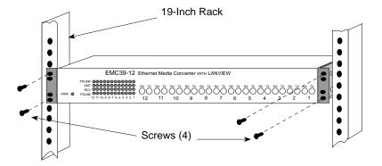
Figure 2-2 Installing the EMC39-12 in a 19-Inch Rack
